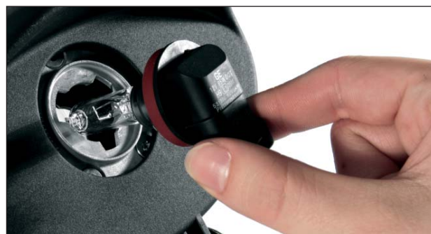
Easy replacement of the H9 bulb without having to open the headlight
